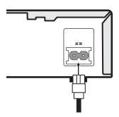
1 Plug the supplied AC power cable into the AC IN inlet and the other end into a standard household power outlet.
